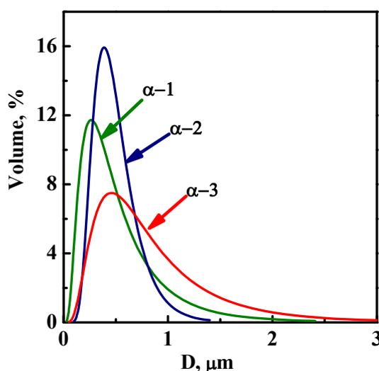
**Figure 3. Volumetric PSD of  $\alpha$ -tocopherol suspensions produced using different expanded liquid solvents:  $\alpha$ -2 Acetone,  $\alpha$ -3 Ethanol and  $\alpha$ -4 isoPropanol.**
