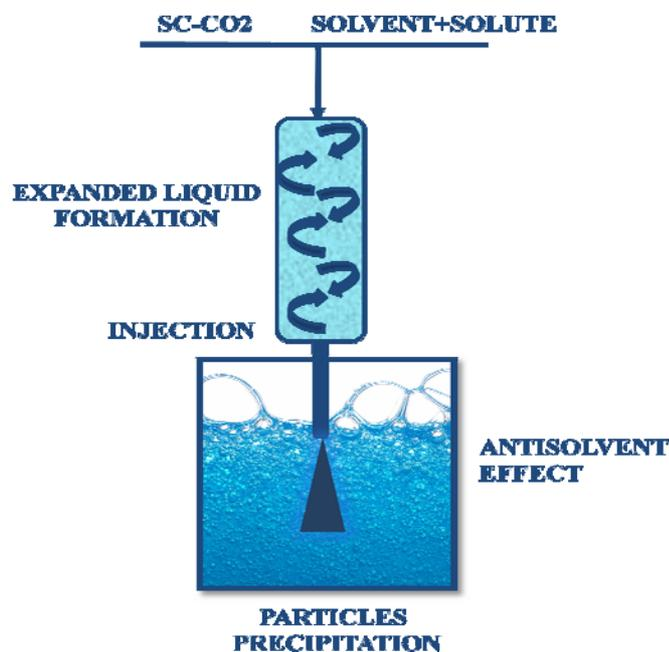
**Figure 1. Schematic representation of SAILA process**
