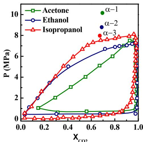
**Figure 2. Vapor-liquid equilibrium curves for the systems acetone-CO<sub>2</sub> (□), ethanol-CO<sub>2</sub> (○), isopropanol- CO<sub>2</sub> (Δ) at 50°C adapted from [10, 11]. Operative points of experiments listed in Table 1 are also reported (●)**
