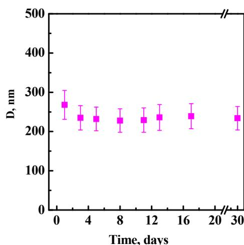
**Figure 4. Suspension stability test:  $\alpha$ -tocopherol mean diameter during 30 days of storage at 4°C.**
